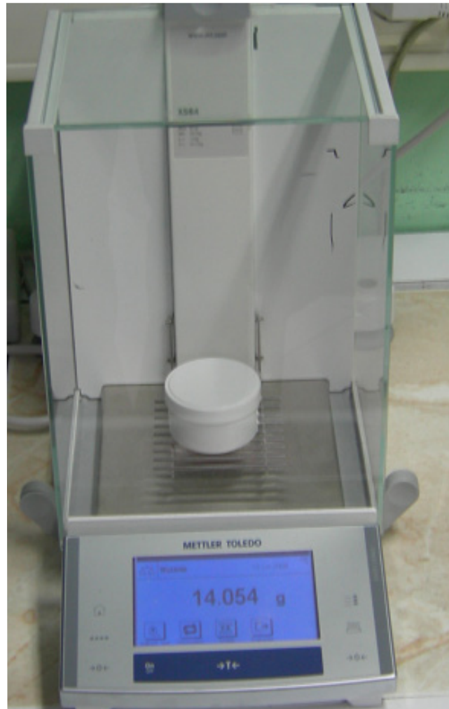
Fot. 2. Measure of the weight of container with the cotton wool.
