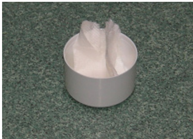
Fot. 1. Container with the cotton wool to accumulate the moisture.
